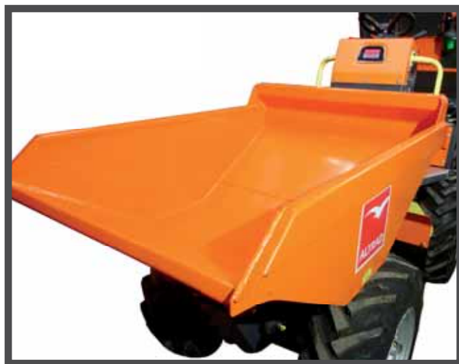
ROBUST, EASY-CLEAN 1000KG CAPACITY SKIP FULLY RETURNED EDGES TO PREVENT DIRT INGRESS
